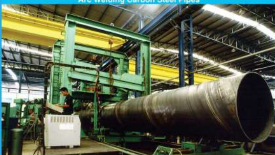
Arc Welding Carbon Steel Pipes
