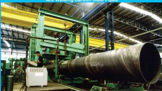
Arc Welding Carbon Steel Pipes
